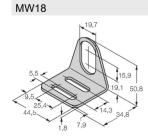
Mounting bracket for threaded barrel sensors; material: Stainless steel A2 1.4301 (AISI 304)
