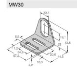
6945005 Mounting bracket for threaded barrel sensors; material: Stainless steel A2 1.4301 (AISI 304)
