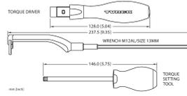
Adjustable torque driver to connect to the 13mm hex. Compatible with redesigned M12 cordsets, M12 Power, and M12 X-code. NOT Compatible with legacy M12 cordsets. Includes (1) adjustable torque driver, (1) adjustment tool, and (1) 13mm forked bit.
