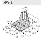
6945004 Mounting bracket for threaded barrel sensors; material: Stainless steel A2 1.4301 (AISI 304)
