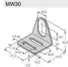
Mounting bracket for threaded barrel sensors; material: Stainless steel A2 1.4301 (AISI 304) BSS-30
