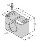
Mounting clamp for threaded barrel
