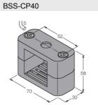
6901318 Mounting clamp for rectangular housings 40 x 40 mm; material: Polypropylene
