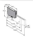
4 digital inputs acc. to EN 60947-5-6 For NAMUR sensors, de-energized contacts or uprox®+ 2-wire DC sensors.
