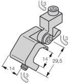
Mounting bracket for mounting magnetic field sensors on tie-rod cylinders; cylinder diameter 40... 125 mm; material: Aluminum
