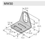
6945005 Mounting bracket for threaded barrel sensors; material: Stainless steel A2 1.4301 (AISI 304)
