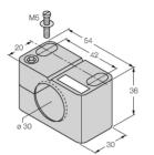
Mounting clamp for threaded barrel
