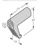
Mounting bracket for mounting magnetic field sensors on tie-rod cylinders; cylinder diameter: 63...160 mm; material: Die-cast Zinc
