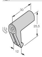
Mounting bracket for mounting magnetic field sensors on tie-rod cylinders; cylinder diameter: 32...100 mm; material: Die-cast Zinc
