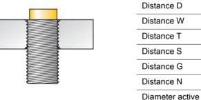
All non-flush mountable uprox®+ threaded barrel sensors can be screwed to the upper edge of the barrel. In this mounting position, the sensor operates safely with a 20 % reduced switching distance.
