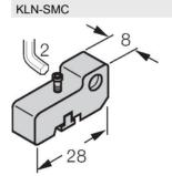
Mounting bracket for mounting magnetic field sensors on SMC cylinders; clamping width 4 mm; material: Anodized aluminum
