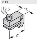
Mounting bracket for mounting magnetic field sensors on profile cylinders (IMI Norgren); cylinder diameter: 32...100 mm; material: Anodized aluminum
