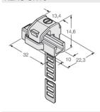
Mounting bracket for mounting magnetic field sensors on round cylinders; cylinder diameter: 63...130 mm; material: PA 6I/6T / nickel silver; fire-hazard classification acc. to UL94 KLRC-UNT4
