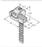
Mounting bracket for mounting magnetic field sensors on round cylinders; cylinder diameter: 63...130 mm; material: PA 6I/6T / nickel silver; fire-hazard classification acc. to UL94
