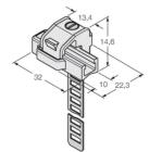
Mounting bracket for mounting magnetic field sensors on round cylinders; cylinder diameter: 25...63 mm; material: PA 6I/6T / nickel silver; fire-hazard classification acc. to UL94 - V2
