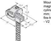
Mounting bracket for mounting magnetic field sensors on round cylinders; cylinder diameter: 25...63 mm; material: PA 6I/6T / nickel silver; fire-hazard classification acc. to UL94 - V2
