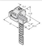
Mounting bracket for mounting magnetic field sensors on round cylinders; cylinder diameter: 63...130 mm; material: PA 6I/6T / nickel silver;
