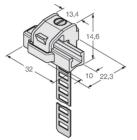
Mounting bracket for mounting magnetic field sensors on round cylinders; cylinder diameter: 25...63 mm: material: PA 6I/6T / nickel silver: fire-hazard classification acc. to UL94
