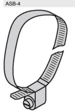
Clip collar for mounting brackets for magnetic field sensors on round cylinders; cylinder diameter: 28... 39 mm; other lengths are available under designations ASB-1 to ASB-9
