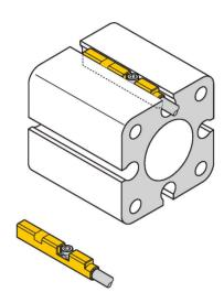
out of the thread and hits the upper grooves with the wings. The sensor is thus pressed down and locked. Use a 1.5 mm Allen key to fasten the screw with a quarter turn. A fixing torque of 0.2 Nm is sufficient for safe mounting without damaging the cylinder. Cable clips are included in the scope of delivery. They enable smooth cable routing in the groove. Mounting accessories for other cylinder sizes have to be ordered separately.
