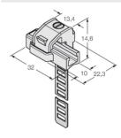
Mounting bracket for mounting magnetic field sensors on round cylinders; cylinder diameter: 130... 250 mm; material: PA 6I/6T / nickel silver; fire-hazard classification acc. to UL94 - V2
