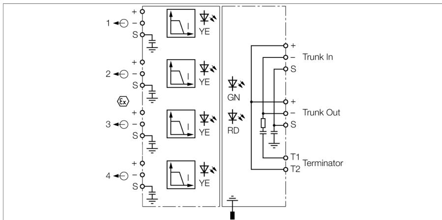
The four-channel multibarrier MBD40-4R/Ex enables the connection of a large number of field devices to one fieldbus in the Ex-area, according to IEC 61158-2.
