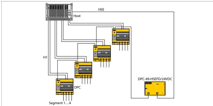
The DPC system (Diagnostic Power Conditioner) is a power supply system for the installation of FOUNDATION™ fieldbus H1 segments. It provides extensive diagnostic options for monitoring FOUNDATION™ fieldbus segments and thus supports plantwide asset management.
