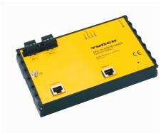
The DPC system (Diagnostic Power Conditioner) is a power supply system for the installation of FOUNDATION™ fieldbus H1 segments. It provides extensive diagnostic options for monitoring FOUNDATION™ fieldbus segments and thus supports plantwide asset management.
