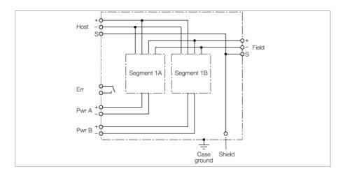
The DPC system (Diagnostic Power Conditioner) is a power supply system for the installation of FOUNDATION™ fieldbus H1 segments.
