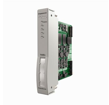
The input module TI40Ex is used for the connection of 2, 3 and 4-wire temperature probes of the types Pt100, Pt200, Pt500, Pt1000, Ni100 and CU100, as well as for the connection of thermocouples of the types B, E, D, J, K, L, N, R, S, T and U. The module can also be used for the measurement of low voltages (-75...+75 mV, -1.2...+1.2 V) and resistance measurements (0...30 Ω, 0...300 Ω, 0...3 kΩ)
