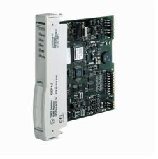
The GDP1,5-FW1.7.6 gateway serves to connect the *excom*® system to PROFIBUS-DP networks. Connections to the PROFIBUS-DP can be established via fiber optics or with copper cables. When using copper cables it is required to use a segement coupler (RS485-IS coupler) on the PROFIBUS-DP side to ensure explosion protection.
