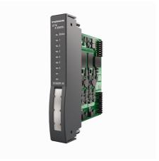
The relay module DO60R-N is used for the connection of non-intrinsically safe actuators such as valves or indicator lights.
