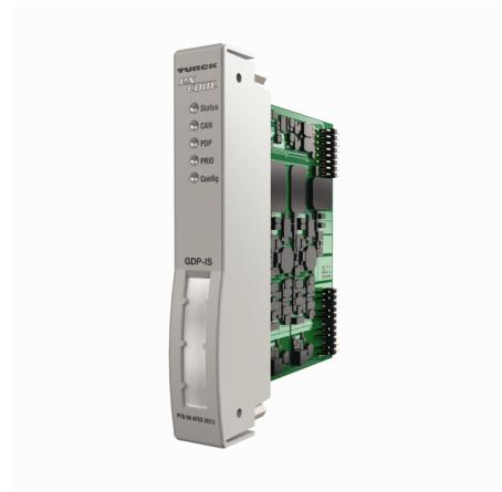
The GDP-IS gateway serves to connect the excom® system to PROFIBUS-DP networks. Connection to the PROFIBUS-DP is established via optical fibers or copper cables. When using optical fibers for data transmission, an optocoupler pair must be installed between wired and optical PROFIBUS which also adapts the level to the IS layer. When using copper cables a segment coupler (RS485-IS coupler) must be installed to ensure explosion protection.
