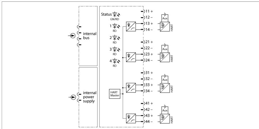
The input module AIH41-N is used for the connection of 4-wire transducers (passive input = sink mode / transducer active).
