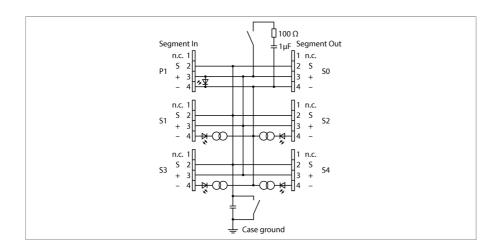
The 4-channel junction box JBBS-49SC-T435 is designed for FOUNDATION™ fieldbus systems.
