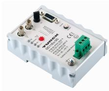
The optocoupler OC11Ex/3G.2 converts the PROFIBUS-DP signals into optical signals. The bus signals can therefore be transmitted from the safe area to the Ex area over long distances without potential or interference. When using fiber-optic cables, the maximum baud range is 2500 m for OM1 (62.5/125-µm) cables and 1500 m for OM2 (50/125-µm) cables.
