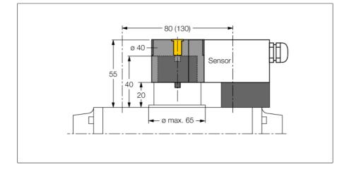
Mounting kit for larger rotary actuators: Spacer plate and snap ring Ø: max. 65 mm Hole pattern on flange surface: 30 × 80 mm (30 × 130 mm) Connection shaft (shaft peg) height 20 mm / Ø max. 40 mm Included in delivery: 1 spacer plate Ø 20 mm (POM) 1 spacer ring Ø 20 mm (PP-GF30)
