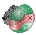
The left figure shows how the read/write head must be aligned towards the data carrier. As an example here the read/write head TNSLR-Q42TWD-H1147 is shown (instructions valid for all suitable read/write heads)
