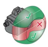
The left figure shows how the read/write head must be aligned towards the data carrier. As an example here the read/write head TNSLR-Q42TWD-H1147 is shown (instructions valid for all suitable read/write heads).
