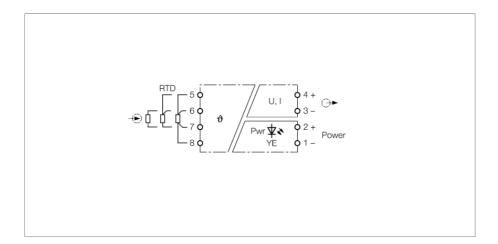
The 1-channel temperature measuring amplifier IMS-TI-Pt100/24V is designed to evaluate the temperature-dependent changes of Pt100 RTDs, to isolate them galvanically and to output them as temperature-linear voltage or current signals of 0...10 V, 0...20 mA or 4...20 mA.
