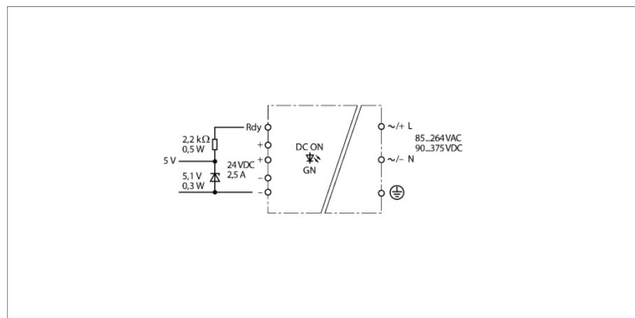
The IM82-24-2.5 power supply unit is designed for DC consumers, in particular for the supply of switching and monitoring devices of the TURCK IM, IME, IMS and IMC series.
