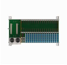
The MT16-2G module rack consists of a back-plane, two PS-F24Ex mains filters and the actual rack system. It can accommodate 2 gateways, 2 power supply units as well as 16 I/O modules. Up to 128 binary inputs/outputs or 64 analog inputs/outputs resp. a mix of both can be connected to it. Two PS-F24Ex mains filters are mounted on the module rack. The mains filters filter the 24 VDC voltage and protect against induced interference in the supply cable
