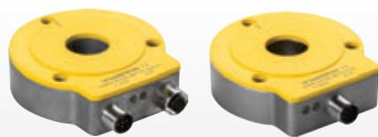
TURCK's Rotary Inductive Analog Sensor operation is based on the RLC (Resistance Inductive Capacitance) principle and incorporates an advanced microprocessor and precisely positioned emitter and receiver coils on a printed circuit board.
