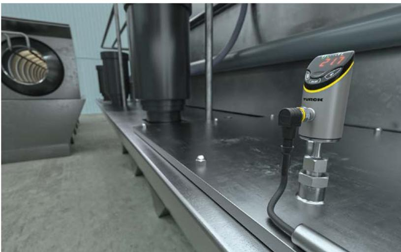
Temperature measurement on drum washers
