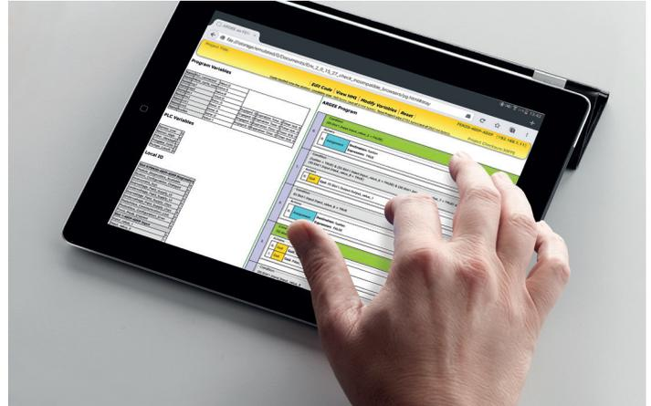
FLC can be used as a local backup for a PLC. If the PLC loses power or connection, FLC technology can do one of two things: either take over the application and run it from the block, or take over the application and safely shut down the process. This can help avoid downtime and troubleshoot where a problem exists on the line.
