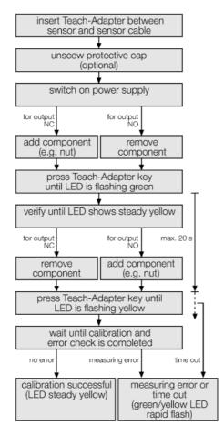
The measuring signal in the sensor is influenced by the diameter and the material characteristics of the center bolt, but also by the cover of the sensitive area. Therefore each sensor has to be conditioned to the operating environment, i.e. to the applied sleeves or protective caps and the target (nut, sleeve etc.) In order to calibrate a sensor, the teach adapter VB2-SP1 made by Turck is needed.
