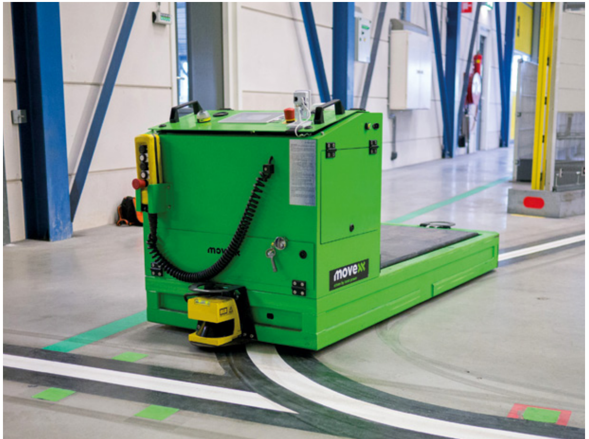
RFID tags that provide the AGV with position information are embedded in the floor at crossings and other key points
